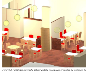
Figure 8.8 Partitions between the diffuser and the closest seats protecting the customers from drafts.
