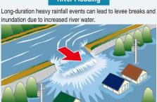
If it rains heavily and the river level rises beyond the drainage capacity of a waterway or a sewer system, rainwater will overflow
