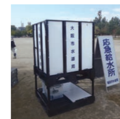
Temporary water storage tank (1 t)
