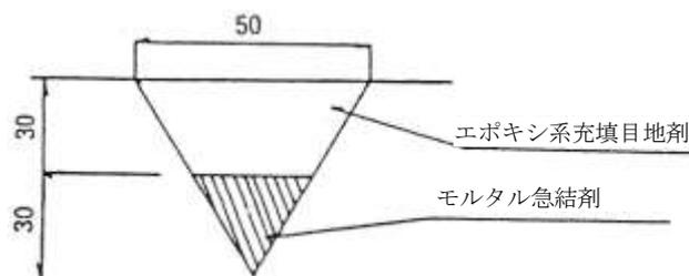
$$\begin{aligned} \text{漏水状態} \left\{ \begin{array}{l} \text{モルタル急結剤} \\ \text{エポキシ系充填目地剤} \end{array} \right. & \quad W_1 = 0.03 \times 0.025 \times \frac{1}{2} \times 1.0 \times 2.9 \times 10^3 \times 1.2 = 1.31 \text{kg/m} \\ & \quad W_2 = (0.025 + 0.05) / 2 \times 0.03 \times 1.0 \times 1.65 \times 10^3 \times 1.15 \\ & \quad = 2.13 \text{kg/m} \end{aligned}$$
